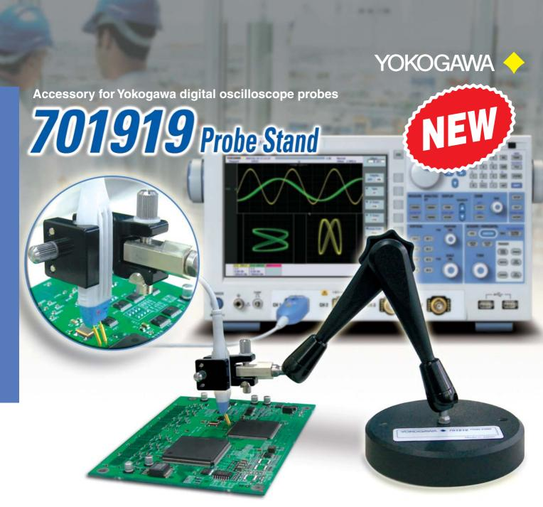
Using oscilloscope probes on today's cramped high-density circuit boards can be challenging. Using a probe stand with a flexible arm and a heavy base to hold and stabilize probes can dramatically simplify circuit board testing.
